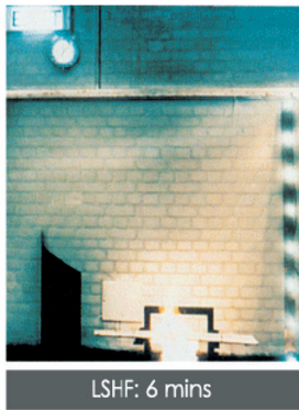
Comparisin between traditional PVC & Low Smoke Halogen Free Cables when tested in accordance to IEC 61034
